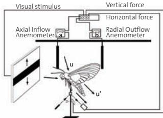
Figure 1. Air flow measurements around a flying insect.
